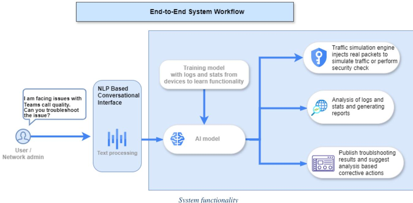
As depicted in the above flowchart, the proposed solution involves an AI-based assistant (that could be running on Aruba Central) which is a system capable of following:
